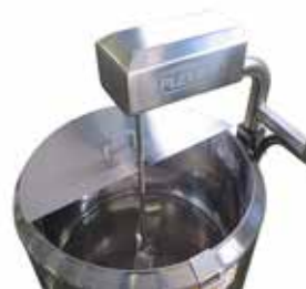
Movable console of the stirrer, two part cover
